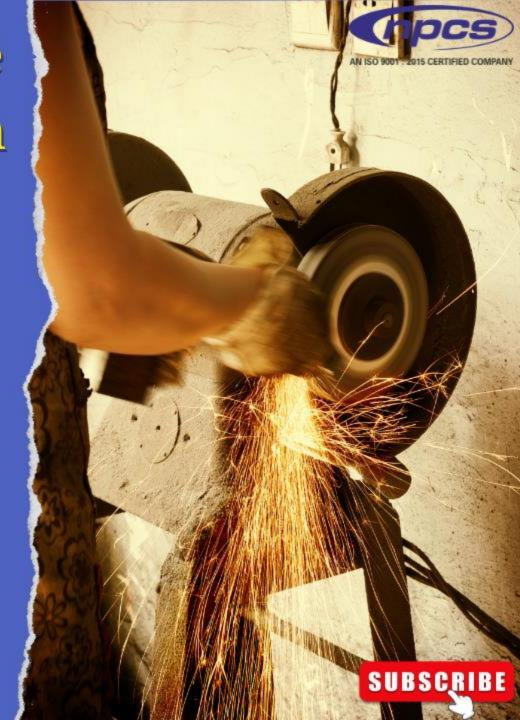
..out faster but they can grind faster than softer ones do. Harder wheels have more edge retention but they will create more sparks when used. Harder wheels are better for rough work while softer ones are good for finishing work.
