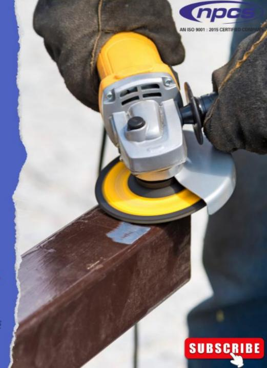
They can be used on almost all metals including aluminum, brass copper etc., ferrous metals such as iron etc., non-ferrous metals such as aluminum bronze etc. They are used in grinding of molds, dies,..
